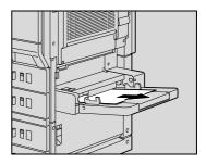
If misfed paper cannot be pulled out, pull the lever for the sliding plate of the bypass tray, and then pull the sliding plate toward you.
