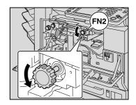
If the punch unit is installed, pull out the hole-punch waste container.
