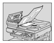
6 Return the document guide lever to its original position, and then close the misfeed-clearing cover.
