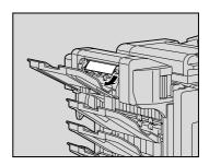
4 Open the misfeed-clearing door, and then pull out any misfed paper.
