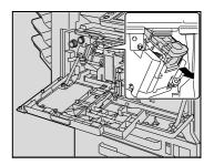
12 Raise the shutter of the staple cartridge holder, and then pull out one sheet of staples.
