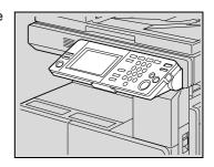
To adjust the control panel to an even steeper angle, pull the control panel release lever toward you, and then push down on the control panel.
