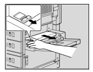
Press down on the sliding plate with your left hand and carefully pull out any misfed paper.
