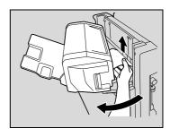
10 Raise the copy output tray, and then push down the staple cartridge holder and remove it.
