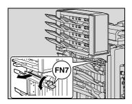
4 Pull handle FN8 to open the misfeedclearing door.
