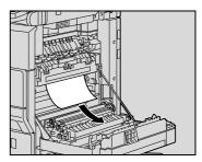
Carefully pull out any misfed paper around the image transfer roller.
