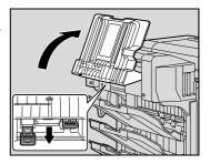
11 Raise the shutter of the staple cartridge holder, and then pull out one sheet of staples.
