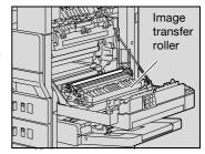
3 Open the fusing unit guide.
