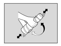
Insert the toner bottle into the toner hopper with the label on the bottle facing up.
