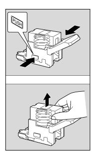
3 Remove the empty staple cartridge from the staple cartridge holder.
