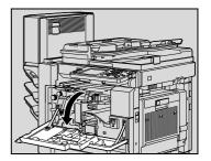
Pull out the hole-punch waste container.
