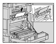
Open the switching guide, and then carefully pull out any misfed paper in the switchback unit.
