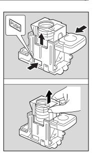
4 Remove the empty staple cartridge from the staple cartridge holder.
