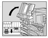
Press in the area marked "PUSH" to unlock the staple cartridge holder.
