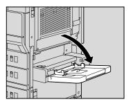
Pull up the lower right-side door release lever, and then open the lower right-side door of the paper feed unit indicated in the touch panel message.
