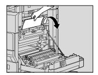
Decreased copy quality may result if the surface of the image transfer roller is touched. Be careful not to touch the surface of the image transfer roller.
